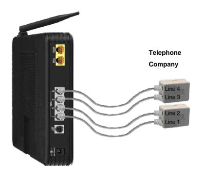
Use the telephone line cords to connect the telephone lines to the **IG7600**.
